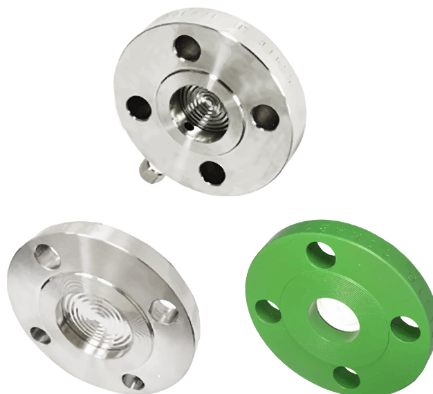
Top: Flanged connection with flush port Left: Flanged connection - welded Right: Flanged connection - screwed + PTFE coating
