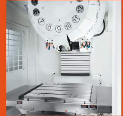
Tapping Center Z axis - Bellows with Lamella
